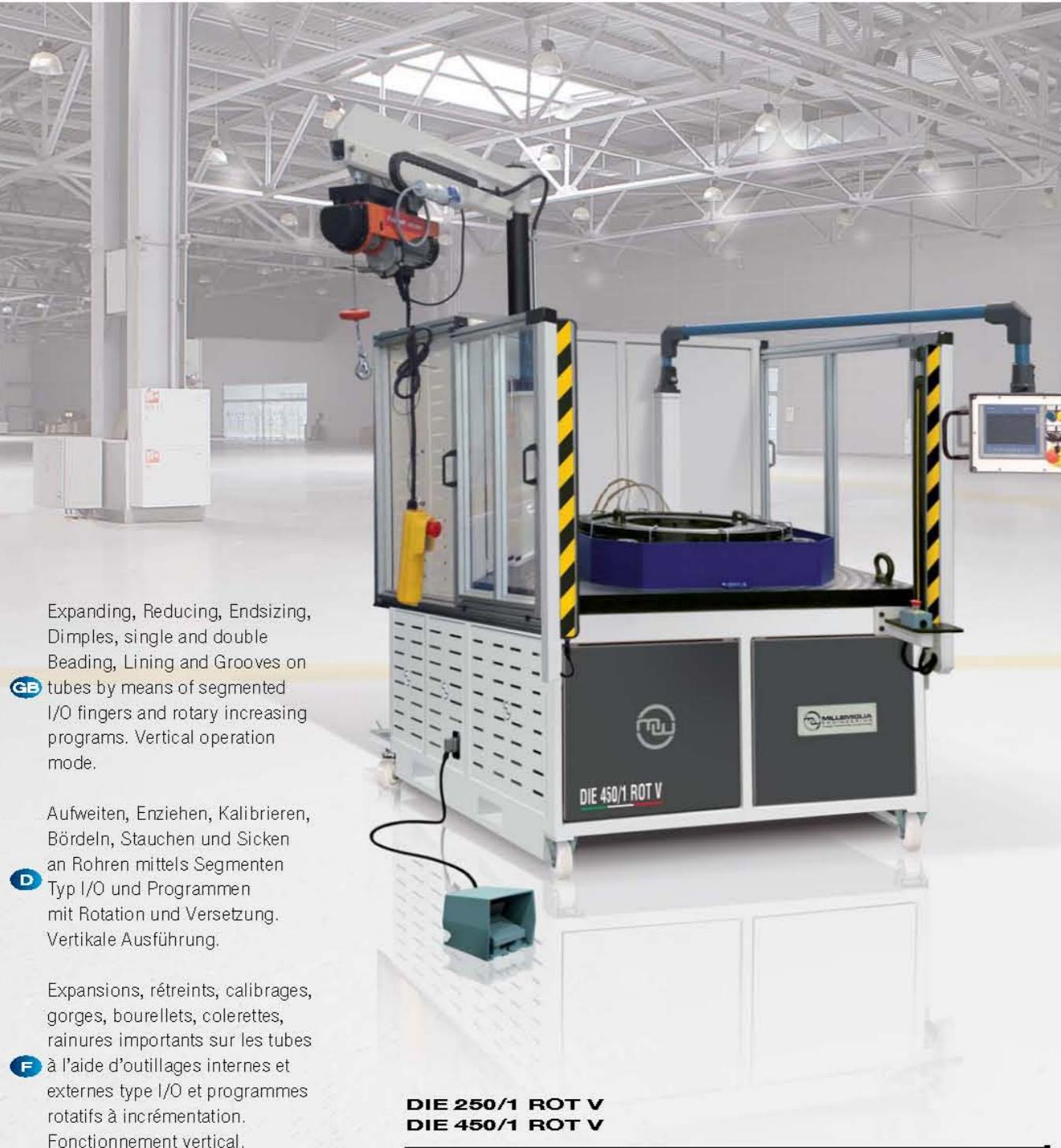
Expanding, Reducing, Endsizing, Dimples, single and double Beading, Lining and Grooves on tubes by means of segmented I/O fingers and rotary increasing programs. Vertical operation mode.
